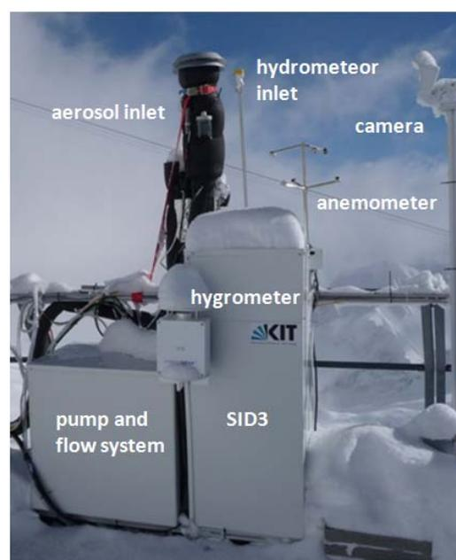
Fig.1: A mobile measurement unit to investigate aerosol cloud interactions located on the roof platform of the Schneefernerhaus (UFS). More instruments are located in the laboratory below.
