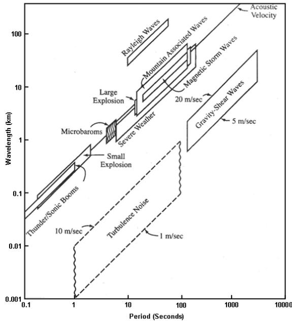
Fig.3: Wavelengths and periods for different infrasonic sources (Figure following Bedard, <http://www.esrl.noaa.gov/psd/programs/infrasound/infrasonic.html> ).
