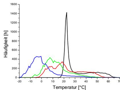
Fig.2: Dispersion of frequency of the average module temperature during one year at the 4 outdoor test sites: Alps (blue), city (green), desert (red) and the tropics (black).
