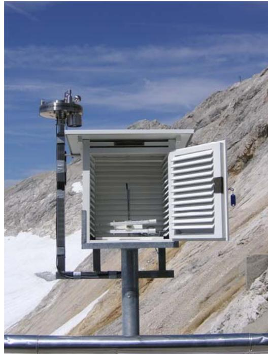
Fig.1: Automatic weather station and conventional weather hut at *Schneefernerhaus* for comparative measurements of daily extreme temperatures
