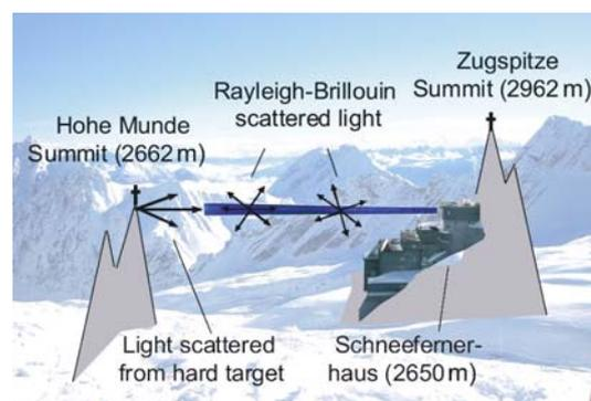
*Fig.1: Rayleigh-Brillouin scattering on a horizontal laser beam path from the UFS towards south.*
