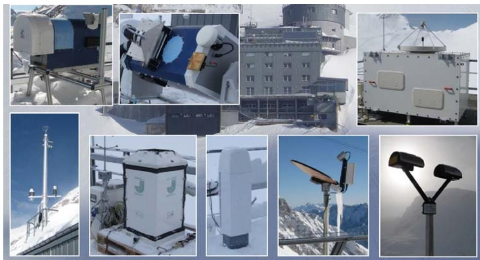
Fig.1: Instruments deployed at UFS during winter 2008/2009. Top from left to right: Microwave profiler HATPRO, 90/150 GHz radiometer DPR, 36 GHz cloud radar MIRA36. Bottom from left to right: 10 m meteorological mast, 2-dimensional video disdrometer, Ceilometer, Micro-Rain-Radar, Parsivel disdrometer.
