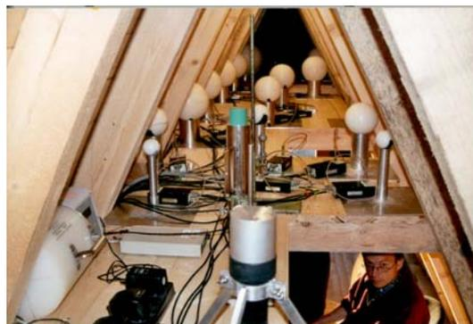
Fig. 1: Bonner Sphere Spectrometer at the UFS.
